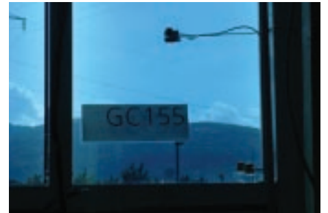
Fig. 1: View through coloured gasochromic glazing, equipped with temperature sensors at Fraunhofer ISE's façade test stand.
