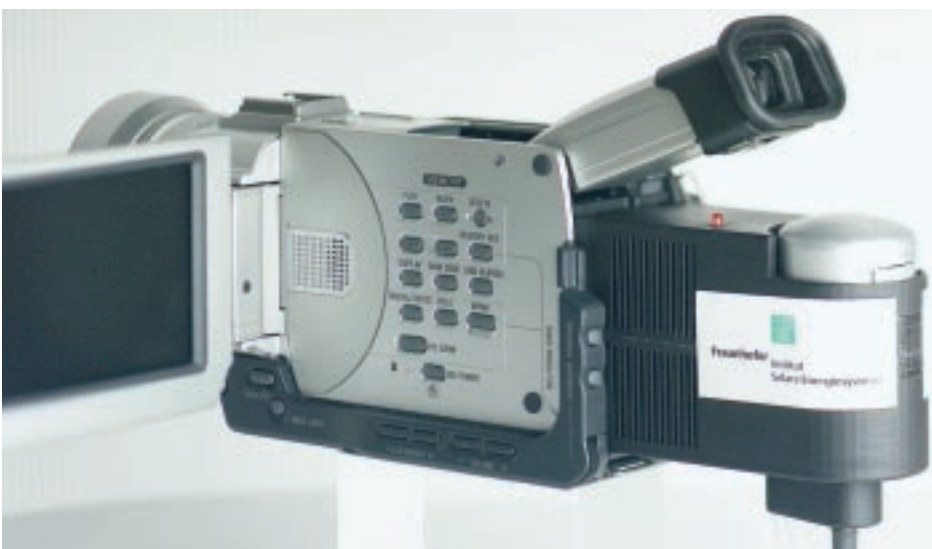
Fig. 1: Commercially available camcorder with a fuel cell system as its power supply. The cylinder to the right is a metal hydride storage capsule for hydrogen.
