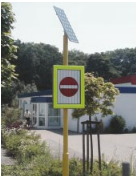
Fig. 1: Photovoltaically powered prismatic display: Rapidly installed, requiring little maintenance and simple to control via the mobile telephone network. (Source: via traffic controlling gmbh).
