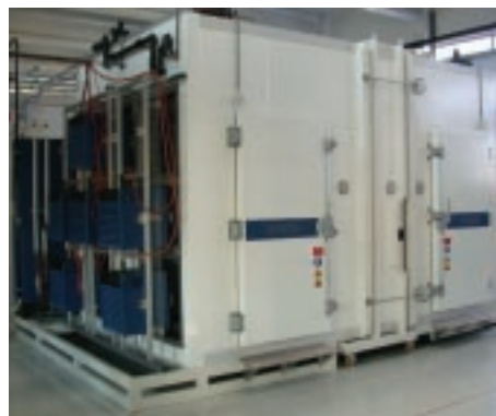
Fig. 2: Dual climatic testing chamber for windows and solar façade components at Fraunhofer ISE.
