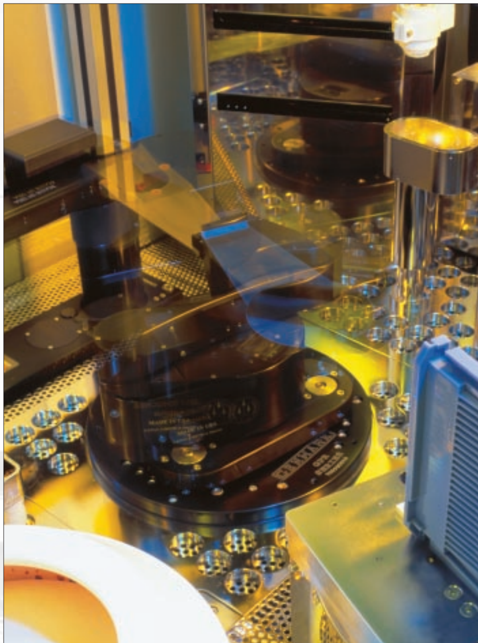
Robot in the automatic lacquering system for silicon wafers in the clean room at Fraunhofer ISE. This system is part of the pilot line to produce highly efficient silicon solar cells.
