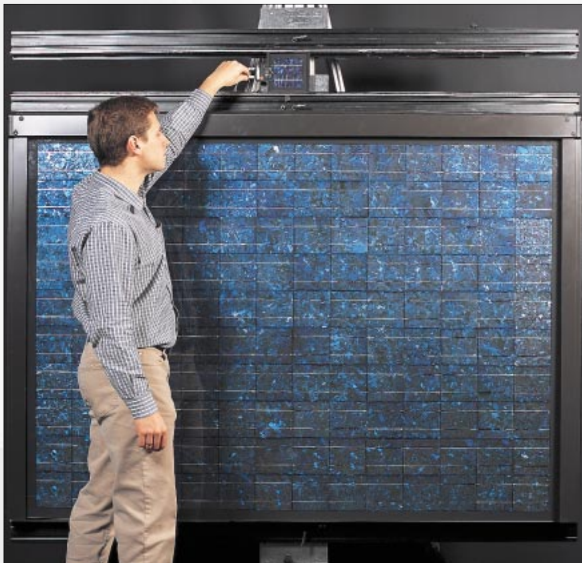
Precision measurement of a 3 m 2 solar module with a rated power of 290 W.
