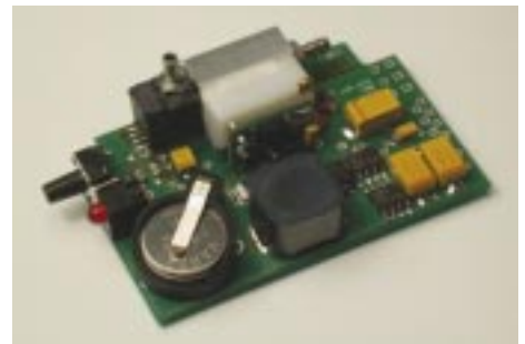
Fig. 1: DC/DC converter for a fuel-cell camcorder. The efficiency value is 97 %. In addition, the circuit includes the hydrogen valve and a button cell for the starting phase. The circuit board is 50 mm long.
