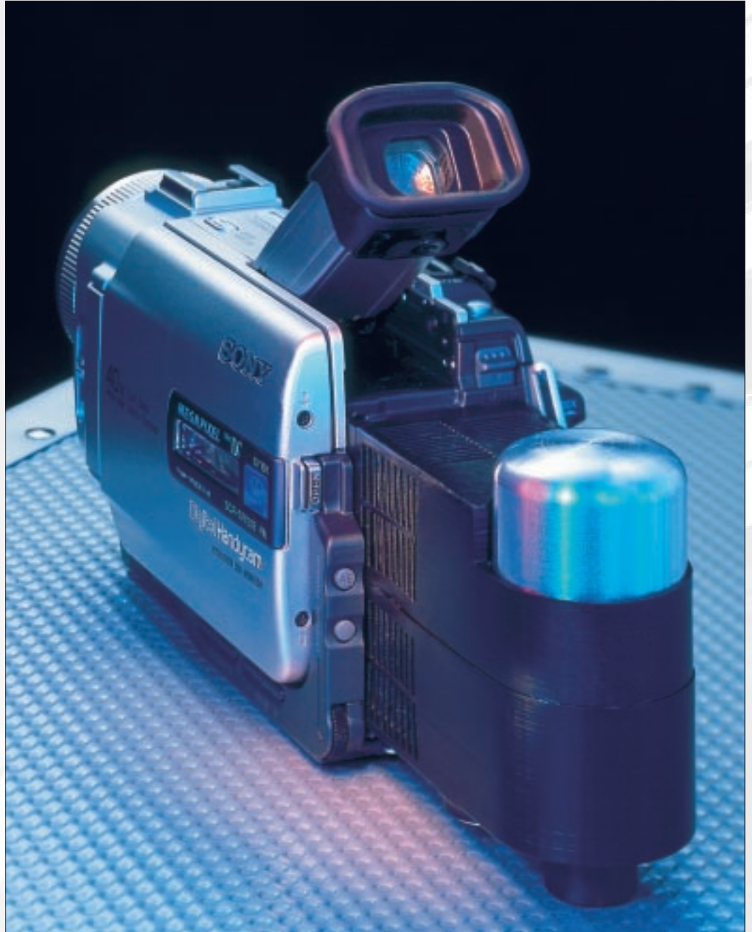
Fuel cell power supply for a digital video camera. The Fraunhofer Initiative on "Miniature Fuel Cells" developed novel bipolar plates, the fuel cell stack, the system controls and processes for series production (see article on p. 54).
