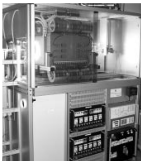
Fig. 3: Equipment to deposit silicon films by the CVD process.
